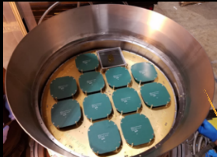
FPU & niobium magnetic shield
