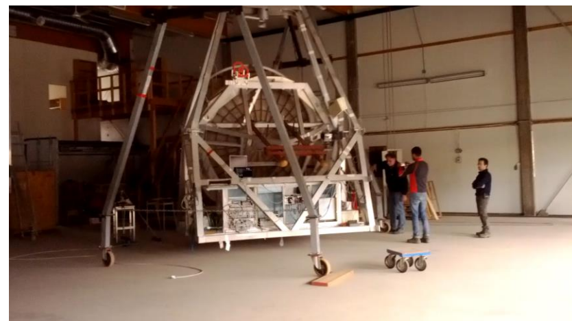
Azimuth Pivot (Boscaleri, IFAC). Same as OLIMPO. Test @ 6 rpm
