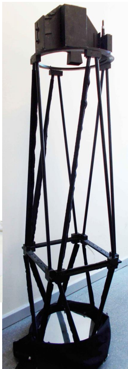
Azimuth Pivot (Boscaleri, IFAC). Same as OLIMPO. Test @ 6 rpm
