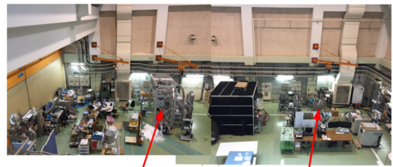
0.1K cosmic ray test cryostat 0.3K utility test cryostat
