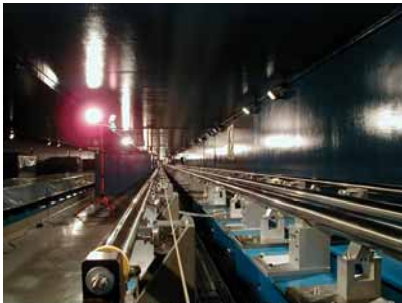
VLTI Delay Lines in the Interferometric Tunnel
