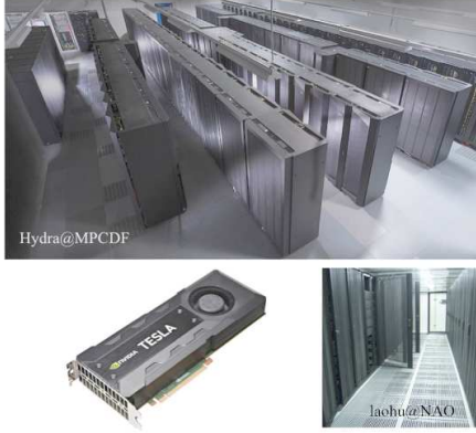
Figure 2.6: Top: The Hydra supercomputer (1.7 PetaFlop/s) operated by the Max Planck Computing and Data Facility is equipped with 676 Kepler K20 GPGPU accelerators (1 PetaFlop/s, bottom left). This supercomputer was used to carry out the DRAGON simulations. Bottom right: The laohu supercomputer of National Astronomical Observatories, Chinese Academy of Sciences in Beijing (96 TeraFlop/s) operated by its Center of Information and Computing is equipped with 64 Kepler K20 GPGPU accelerators. Credit: MPCDF/NAO.
