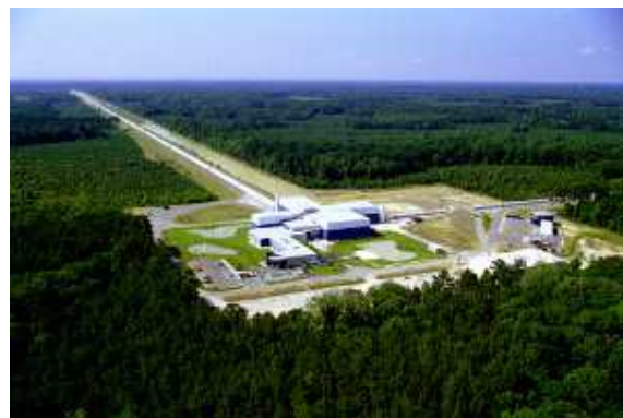
Figure 2.25: Aerial view of the LIGO gravitational-wave detector at Livingston, U.S.A.; the two monitoring arms containing strong laser beams extend to a length of 4 km. Copyright: LIGO Laboratory
