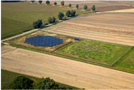
Figure 2.20: The LOFAR antenna array near Unterweilbach is operated by the MPA. It is one of the 6 stations in Germany and 40 stations in the Netherlands that are combined to study the largely unexplored frequency range between 10 and 240 MHz. copyright: Rainer Hassfurter/MPA
