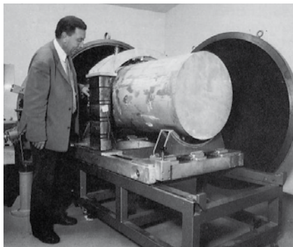
The aluminium cylinder of Joseph Weber's gravitational wave experiment, which was repeated in Munich. In front Heinz Billing, supervisor of the experimental setup at the MPA.
